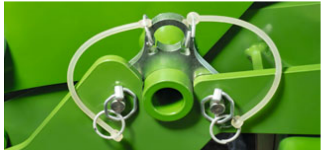
The three easily accessible coupling points of the QuickLink system ensure safe and fast, tool-free coupling and uncoupling.
