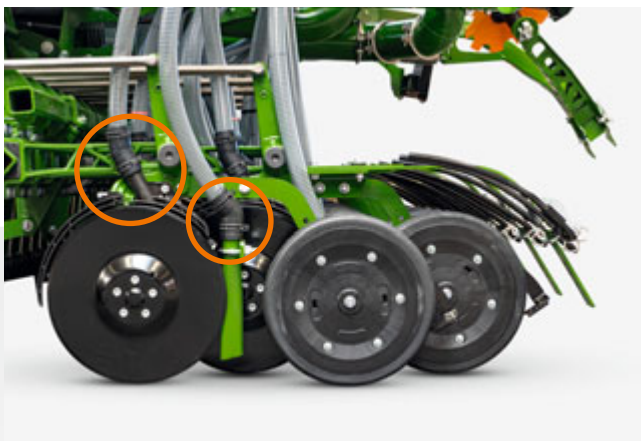
TwinTeC coulters with an additional outlet
