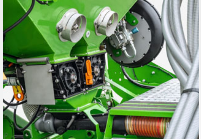
Two metering units for a wide variety of materials
