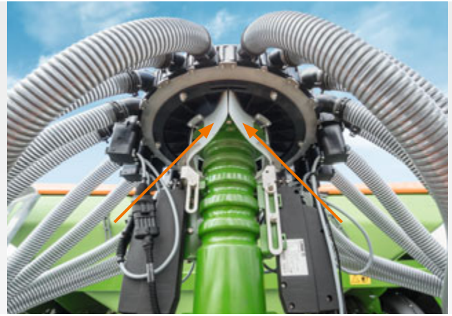
Segmented distributor head with electric half-side shut-off (not activated)
