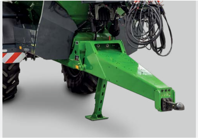
✔ Hitch coupling with K80 ball coupling
