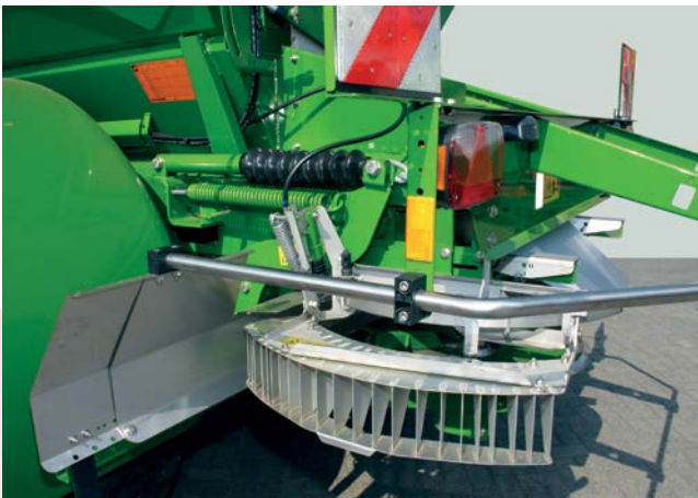
Limiter border spreading system in working position
