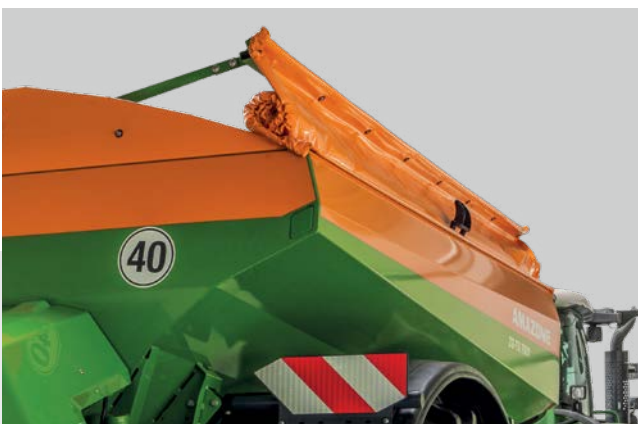
✔ Hydraulically actuated roll-over hopper cover
