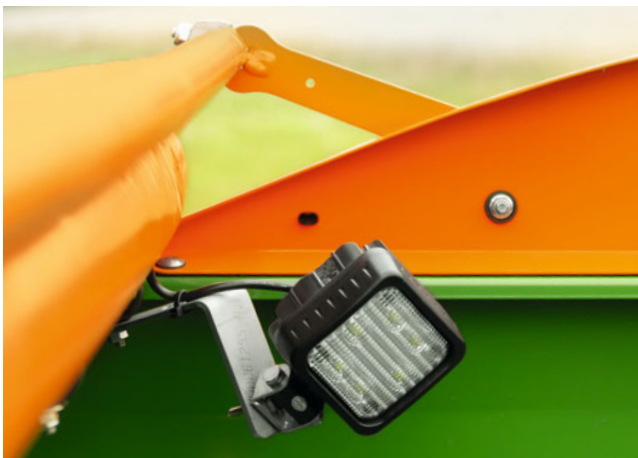
Lighting for the inside of the hopper
